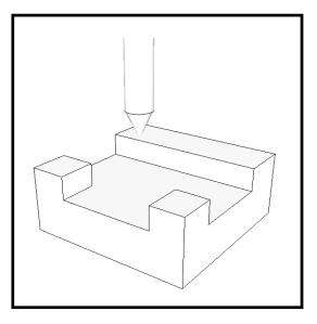
**Step 1:** The print head lays down the first layer of the model. Some printers will lay down a layer that will later be wasted, made from another material. **Step2:** The print head covers each layer with a new layer, building a 3D form from the bottom up.
